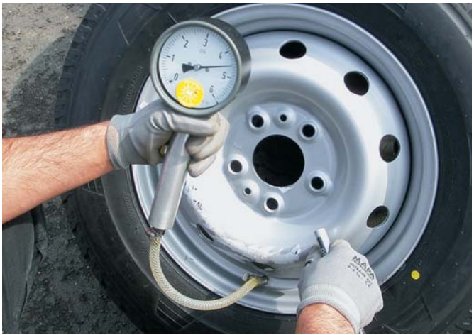
C tires for the Ducato size 215/70 R 15 perform best with an air pressure of 4.5 bar; CP tires can take an additional 1.0 bar.
