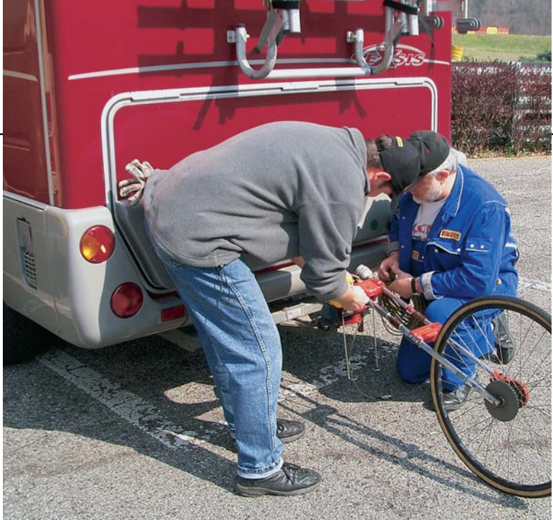
The brake tests use a modern old-timer: the "Preiseler" wheel, which measures the exact speed of the Hymer Exsis.
