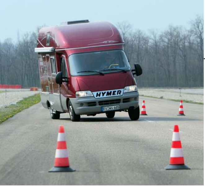
Fast swerving maneuvers may increase the lateral pressure on the caravan; the tires can either reduce the tendency to roll over-or increase it.
