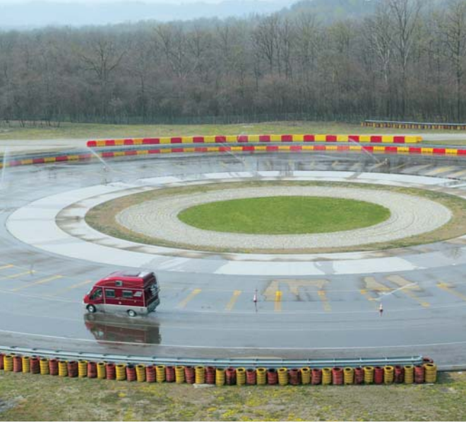
Round and round goes the lateral traction test. The driven time sheds light on the static friction of the tread material compound.
