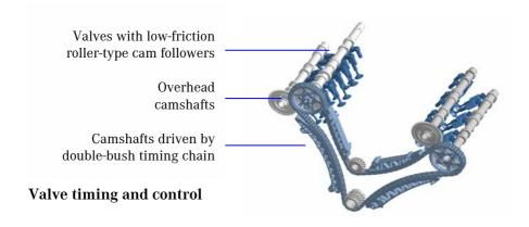
The camshaft bearings are directly integrated into the cylinder heads and cylinder head covers. This new concept not only saves space, but also has acoustic advantages.
