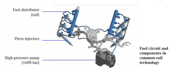
Mercedes engineers have also made improvements to other components of the common-rail system and the injection process:
