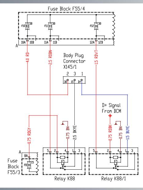
When installing electrical aftermarket equipment with an AMP draw of more than 25A it is necessary to use the optional aux battery 12V/100Ah (CODE E28)
