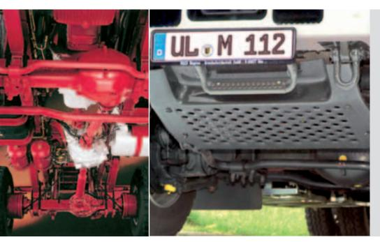
Standard for all all-wheel chassis: The steel protection plate for protecting the radiator and oil sump as well as the robust steel bumper bars
