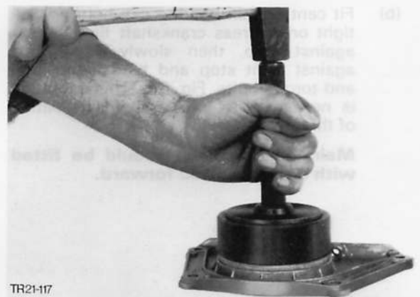
Fig. 71. Press in crankshaft rear oil seal using Special Tool 21-011-A
