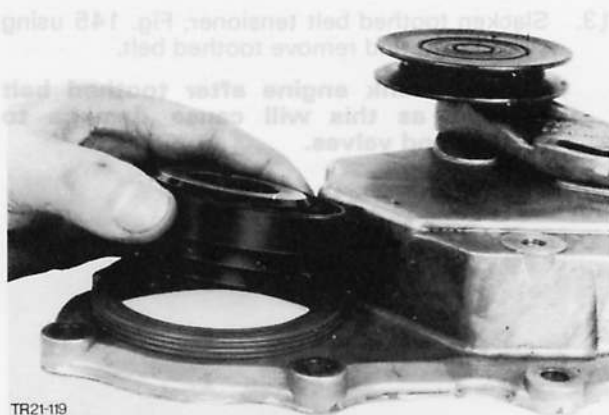
Fig. 148. Fit crankshaft oil seal using Special Tool 21-025
