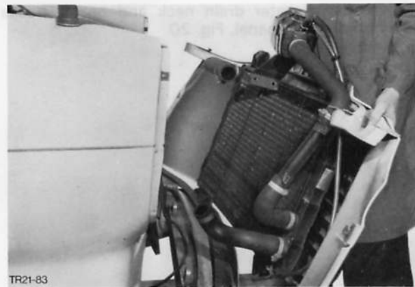
Fig. 17. Remove radiator grille panel complete with radiator, expansion tank and connecting pipe
