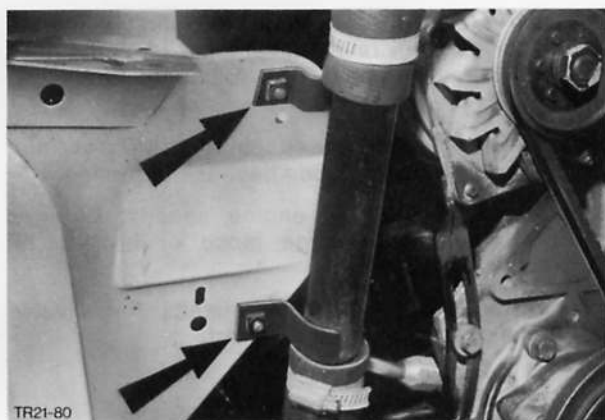
Fig. 14. Unscrew expansion tank connecting pipe
