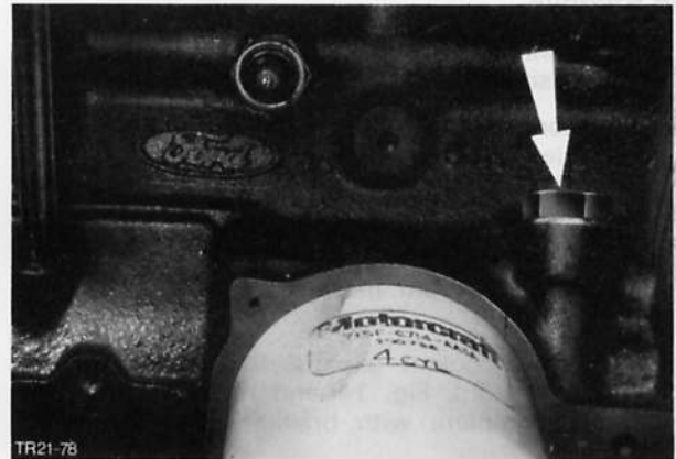
Fig. 11. Relief valve location (vacuum pump removed for clarity)
