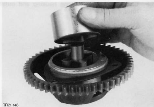
Fig. 170. Insert outer rotor with chamfered side into housing
