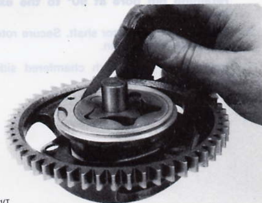
Fig. 173. Measure clearance pump housing/outer rotor
