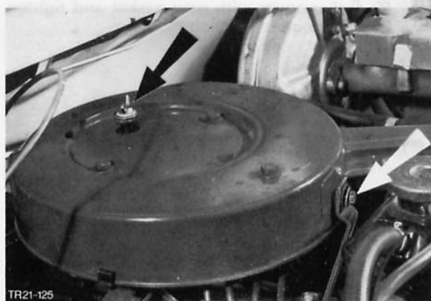
Fig. 110. Fit air cleaner
